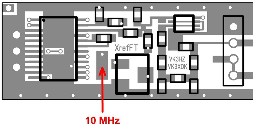
Align the XRef-FT board so the black connector is on top and towards the 4-pin header end. The 3-pin header should be in line with three holes in the board. Note that there is no connector on the Xref board at the 3-pin end – these are all ground pins.
