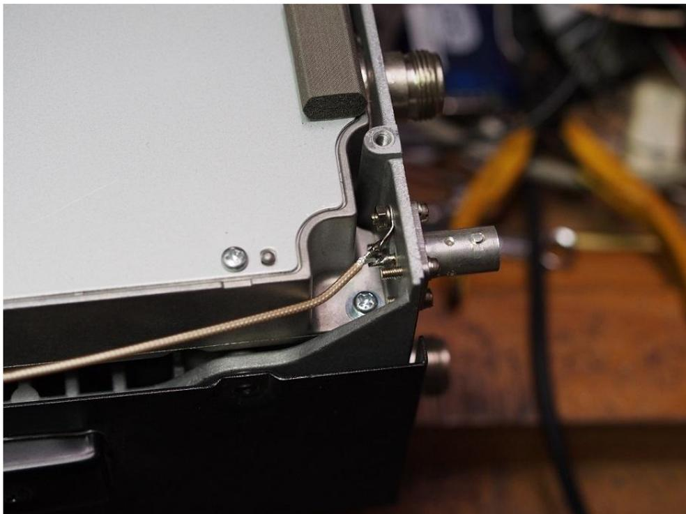
**Figure 6. – Possible 10MHz Input Socket Location**
