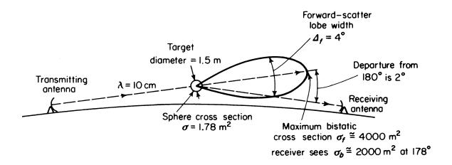
Figure 1: An example of bistatic radar where the transmitter and receiver are close to alignment, copied from Barton<sup>9</sup>
