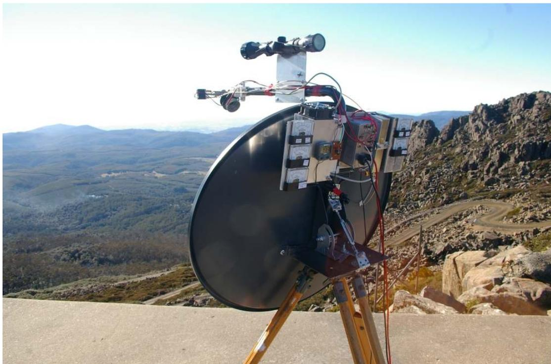
At the Mt Fatigue end, 7 watts was going into a 45 cm diameter dish antenna. The plan was to leave the radio equipment outside in the cold and operate the laptop from within the car. In the event, it was a balmy 18 degrees on the hilltop so the deckchair operating position was adopted.
