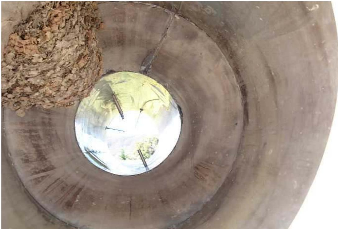
So now he knows that a swallows nest in the feed is worth 2.2dB off the receiver. The nest was carefully relocated and a more secure cover was fabricated to prevent any further invasions. The swallows are probably missing that nice warm feeling they encountered during the recent EME contest.
