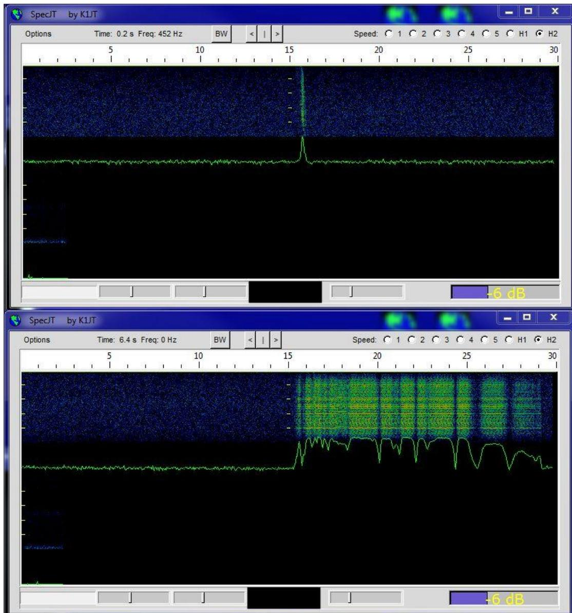
**Fig 1: Concurrent MS signal on 70 cm (upper) and 2 m (lower)**
