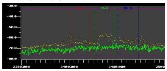
The "grass" is probably WiFi, cordless phones and the like, while the broadband interference is probably an AV sender. It clearly shows that the area in which we operate for weak signal operation – 2403 MHz – is being swamped with interference.
