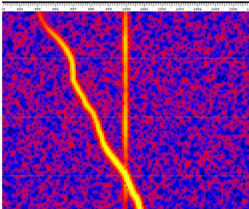
**Spectrum Lab waterfall display showing Doppler Shifted frequency from aircraft as the slanted line and the direct troposcatter signal as the straight line at 1000 Hz.**
