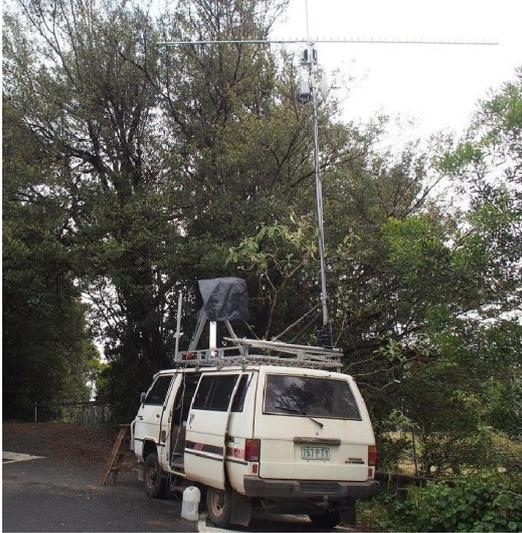
*I parked strategically in order to take advantage as much as possible of a small gap in the foliage, but it meant abandoning the roof-mounted 2.4 GHz array and associated M/H box. The mast with 1296, 5760 and 10368 MHz antennas was looking over some of the immediate vegetation, but the 24 GHz antenna (on tripod under the plastic rain cover) was mostly blocked.*
